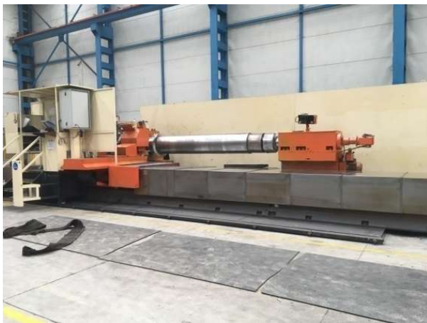
CNC HEAVY DUTY LATHE ( WITH C AXIS ) D.S. WOHLBERG Length: 8.000mm, Dia.: Ø1.400mm
