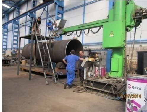
COLUMN & BOOM SYSTEMS AND ROTATORS 1 Piece of 4.000x4.000mm Column & Boom 1 Piece of 3.000x3.000mm Column & Boom
