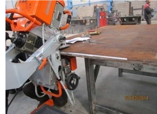
BEVELLING MACHINES ( X and V bevelling thickness is up to: 70m)
