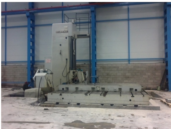
CNC BOHRWERK HEYLIGENSTAEDTH X: 4.000mm, Y: 2.200mm, Z: 800mm
