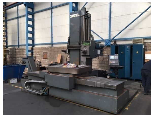
CNC BOHRWERK CASTEL GREEN X: 2.100mm, Y: 1.500mm, Z+W: 1.500mm
