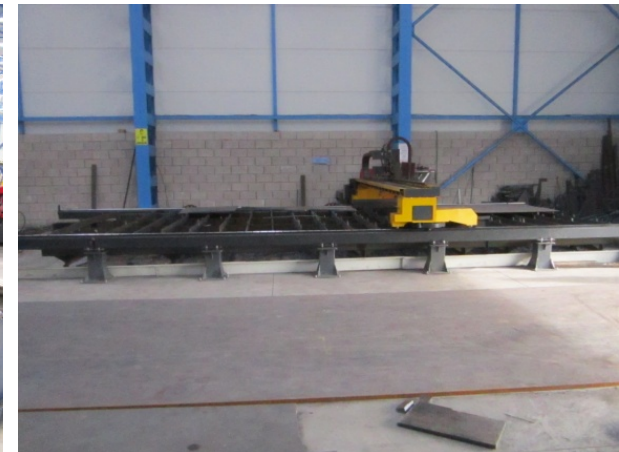
CNC OXY-PLASMA CUTTING - AJIAN X: 8.000 mm Y: 3.000 mm Thickness: 5mm-300mm
