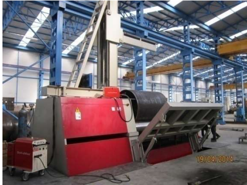
4 ROLL HYDRAULIC PLATE BENDING MACHINE ( 3.100x80mm ) AKYAPAK Bending Thickness: 20.0mm - 80.0mm Bending Dia.: Ø750mm - Ø 5.000mm
