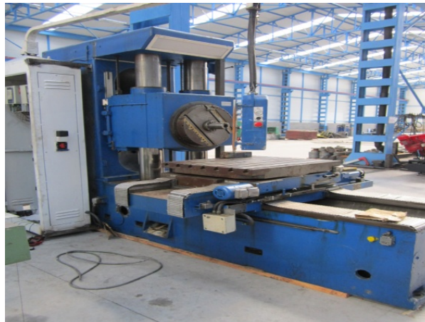
BORING MILL SCHARMANN X:1.200mm, Y:800mm, Z:800mm
