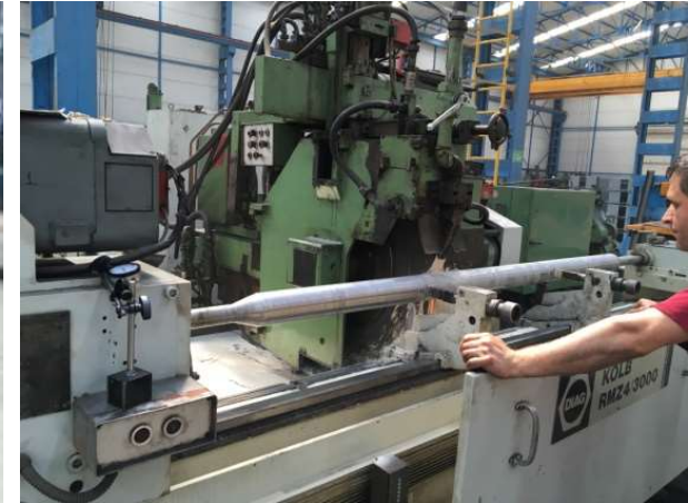
CYLINDRICAL GRINDING MACHINE KOLB DIAG Length: 3.000 mm, Dia.: 500 mm
