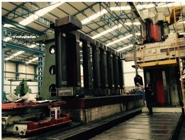
FLOOR TYPE HORIZONTAL BORING MILL PAMA TITAN AFP 180 X:10.500mm, Y:4.000mm, Z+W: 2.200mm
