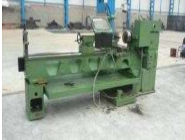
LATHE SN-50 TOS Length: 2.000mm, Dia.: Ø500mm
