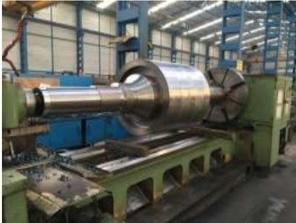
HEAVY DUTY LATHE TOS Length : 3.000mm, Dia.: Ø710mm
