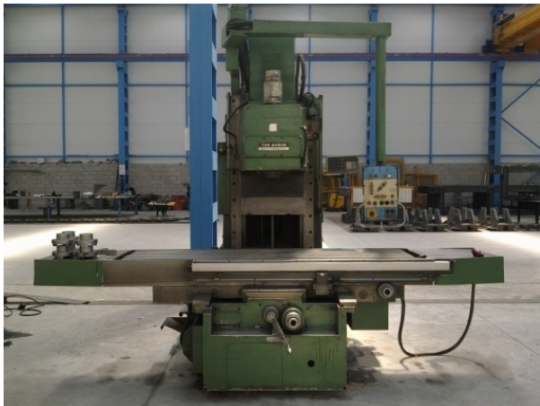
VERTICAL MILLING MACHINE TOS KURIM X: 1.7000 mm, Y: 800 mm, Z: 800 mm
